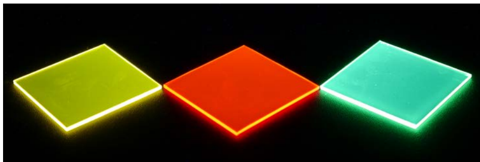
Figure 1. Photos of NOL-containing PMMA plates under a UV irradiation.
