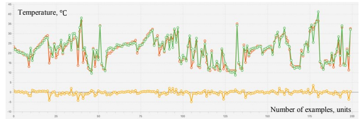
Figure 8. Test set evaluation using neural network model. Green colour indicates T239 sensor's readings. Red curve represents neural network output. Yellow colour stands for network error.
